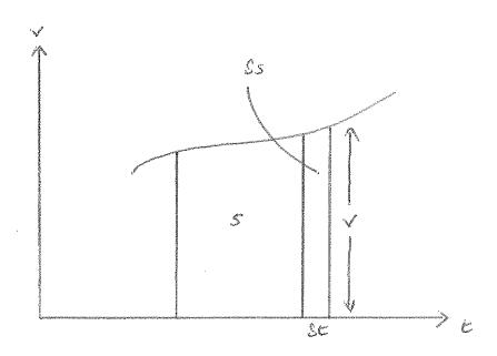
v & s can be interpreted as speed and displacement, but the argument holds for other situations. s is defined to be the area under the curve of v, and, by the first definition of integration,
